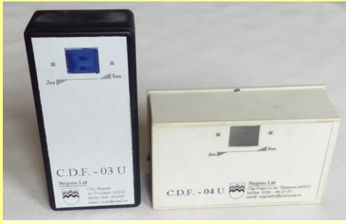
9.15. Four generations of Control Devices of Frequency (CDF 0x) microcomputer Z8 based, for Terapia Cluj-Napoca (2000-2006)
